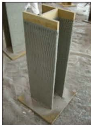
Fig. 3: Carbon fiber hybrid mesh on structural steel piece. Photo courtesy of WIWA GmbH
