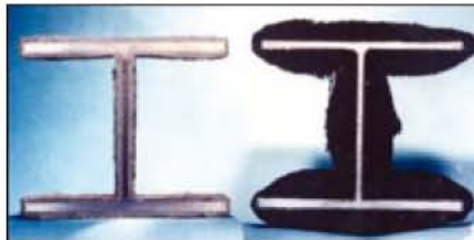
Fig 1: Intumescent coating applied to steel beam (left) and after the coating has been exposed to heat/fire and has expanded (right). Photo courtesy of International Paint
