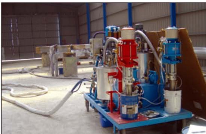
Fig. 4: Units for plural-component application of intumescent. Photo courtesy of WIWA GmbH
